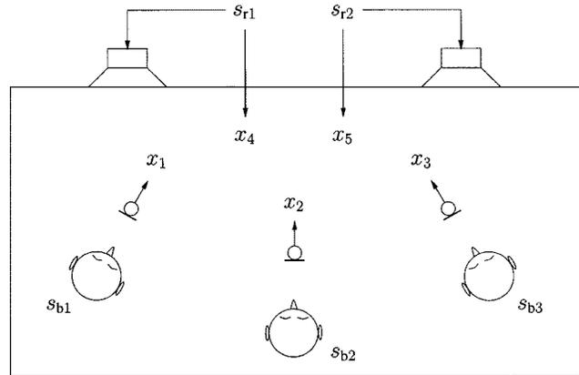
Fig. 1. Teleconferencing setup. Some signals are unknown (speakers) and some signals are known (loudspeaker signals). The loudspeaker signals  $s_{r1}$  and  $s_{r2}$  are directly conveyed to the virtual sensors  $x_4$  and  $x_5$ , respectively.
