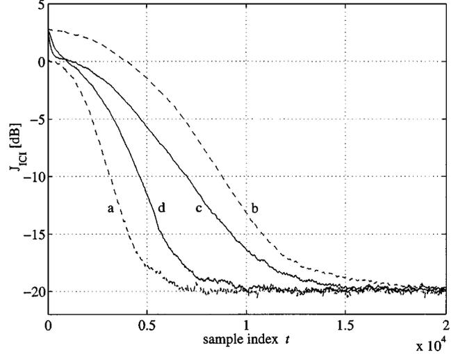
Fig. 4. Separation performance of the combined blind/nonblind separation algorithm averaged over 50 runs. (a)  $M_s = 5$ ,  $M_r = 0$ ,  $M_b = 5$ , (blind only), and  $\mu = 0.004$ . (b)  $M_s = 10$ ,  $M_r = 0$ ,  $M_b = 10$ , (blind only), and  $\mu = 0.002$ . (c)  $M_s = 10$ ,  $M_r = 5$ ,  $M_b = 5$ , and  $\mu_1 = \mu_2 = 0.002$ . (d)  $M_s = 10$ ,  $M_r = 5$ ,  $M_b = 5$ ,  $\mu_1 = 0.003$ , and  $\mu_2 = 0.001$ .
