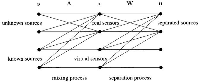
Fig. 3. Incorporation of the known sources as virtual sensors ( $M_r = 2$ ,  $M_b = 2$ ).
