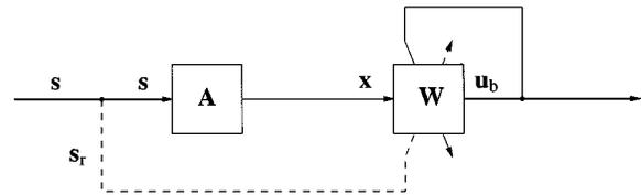
Fig. 2. Basic architecture for a combined blind/nonblind separation algorithm. The dashed line shows the path with the subset of known signals. Discarding this path leads to the more familiar blind-only case.
