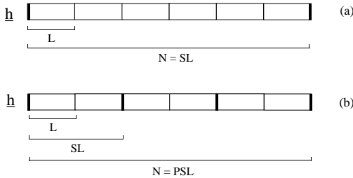
Figure 3: Partitioning of the filter impulse response: (a) no partitioning: P=1, S=6 (b) with partitioning: P=3, S=2 .
