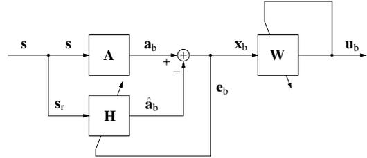
Figure 4: ( $\mathcal{A}4$ ) Combined echo canceller and blind source separation.
