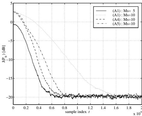
Figure 8: Performance of the combined blind/non-blind separation algorithms averaged over 30 runs. The step-sizes  $\mu$  are individually adjusted so as to result in the same separation degree  $J_\infty(\mathbf{P}_b) = -20\text{dB}$ :  $\mathcal{A}1$ :  $\mu = 0.065$ ,  $\mu = 0.03$ ,  $\mathcal{A}4$ :  $\mu = 0.055$ ,  $\eta = 0.001$ ,  $\mathcal{A}5$ :  $\mu = 0.035$ .
