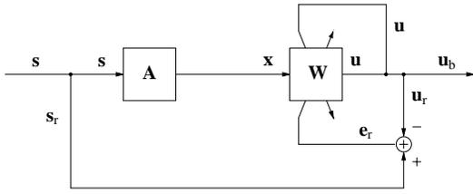
Figure 5: ( $\mathcal{A}5$ ) Combined equalizer and blind source separation.
