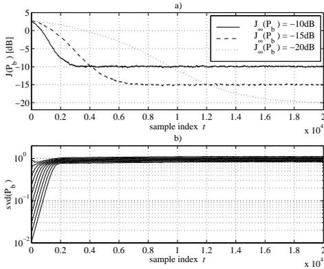
Figure 7: Performance of the blind separation algorithm  $\mathcal{A}1$  for  $M_s = 10$  sources. a) Performance measure  $J(\mathbf{P}_b)$  as described in section 4.1. b) Singular-value decomposition (SVD) of the permutation matrix  $\mathbf{P}_b$  for  $J_\infty(\mathbf{P}_b) = -20\text{dB}$ .
